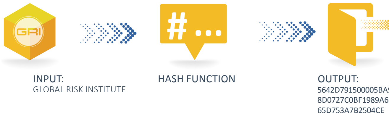
Figure 3. SHA-256 hash function value (output) for the phrase “Global Risk Institute” (input)
