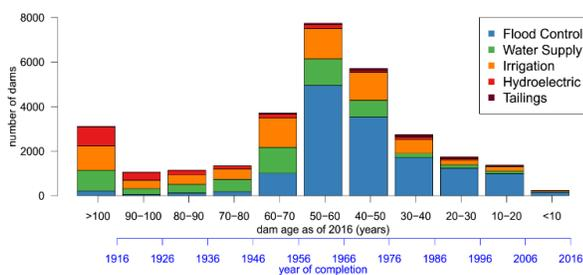
**Figure 1** . Age of dams (from National Inventory of Dams database) with primary uses of flood control, water supply, irrigation, hydroelectric or tailings dams.
