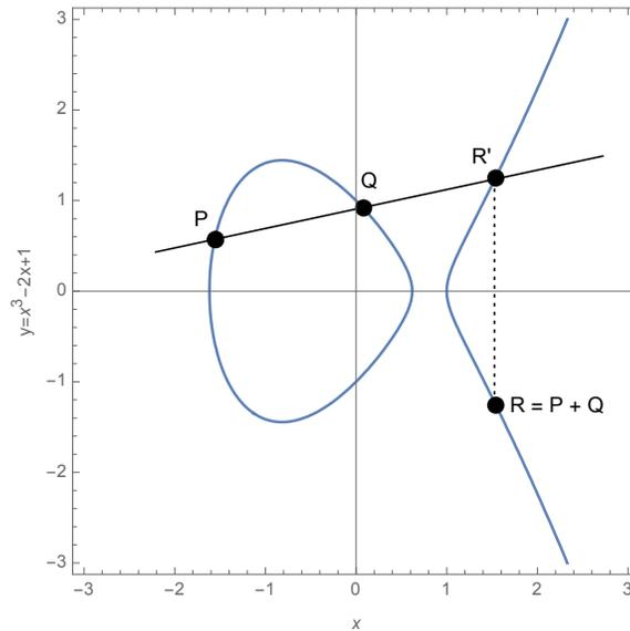
**Fig. 1.** Adding two different points  $P$  and  $Q$  on the elliptic curve  $y = x^3 - 2x + 1$ .
